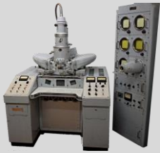
JEOL JXA – 3SM CJ 1963 Acc.Volt. 5-50 kV Max. Resolution 100nm
