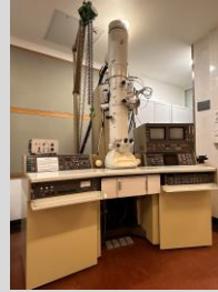
JEOL JEM – 2000FX CJ 1986 Acc.Vol. 80 – 200 kV Max. Resolution 0.25nm
