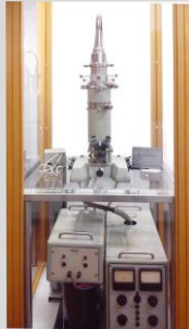
Tesla BS 242 E CJ 1963 Acc.Volt. 35-65 kV Max. Resolution 2.5nm
