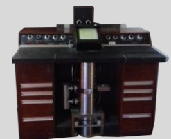
AEI Corinth 500 CJ 1974 Acc.Volt. 20-80 kV Max. Resolution 1nm
