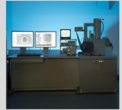
Philips ESEM XL-30 CJ 2002 Acc.Volt. 0.2-40 kV Max. Resolution 3.5nm
