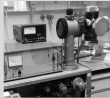
Leybold Heraeus AS 050 Evaporation system CJ 1970
