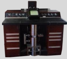
AEI Corinth 500 CJ 1974 Acc.Volt. 20-80 kV Max. Resolution 1nm
