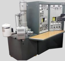
Cambridge Stereoscan Mark II CJ 1972 Acc.Volt. 1-30 kV Max. Resolution 10nm
