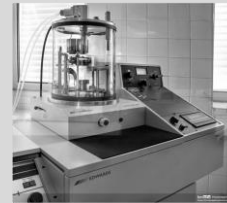
Edwards Auto 306 Turbo Evaporation system CJ 1998
