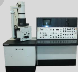
Cambridge Stereoscan 250 MK CJ 1984 Acc.Volt. 0,5-40 kV Max. Resolution 6nm
